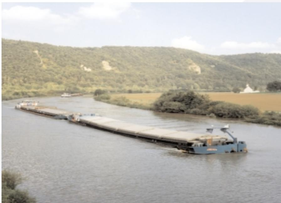
river bends. As a consequence of the common acting of various forces like resistance, centrifugal and steering forces induced by rudder blades, a torque appears that turns the vessel relative to the direction of its motion for so-called drift angle. In case of very long vessels like large pushed trains the width requirements through the curve might be considerably bigger than the total breadth of the vessel.
